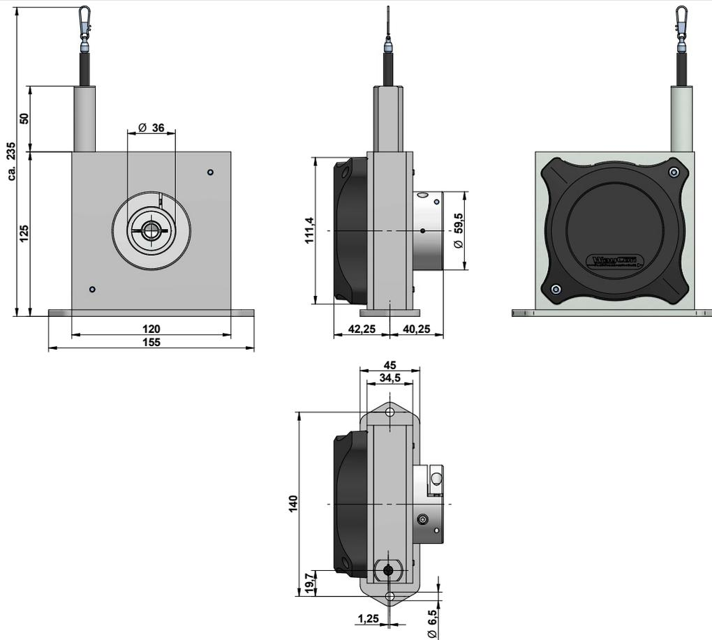
**TECHNICAL DRAWING SX135 MECHANICS MEASUREMENT RANGE UP TO 8 m**
