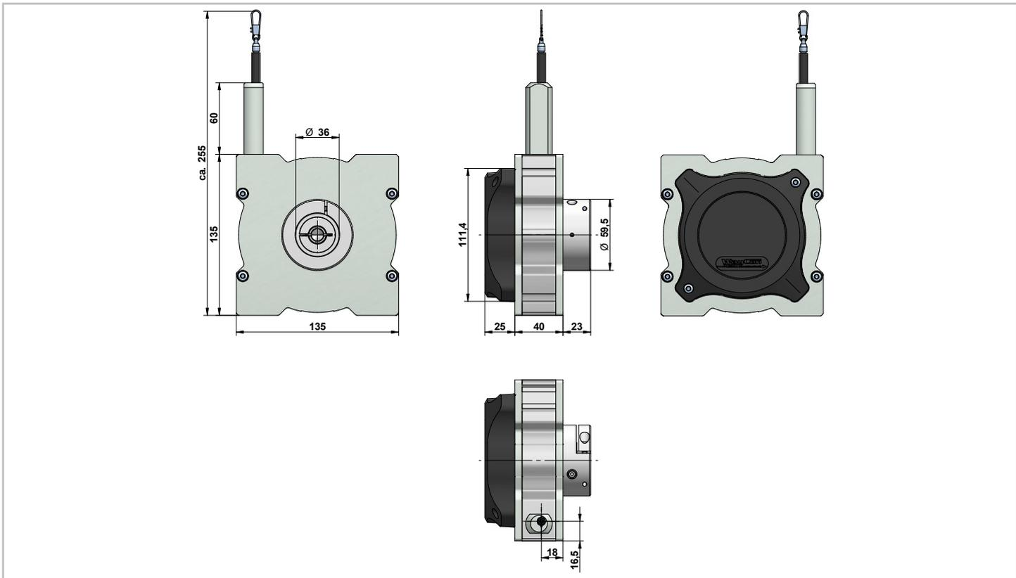
**TECHNICAL DRAWING SX135 MECHANICS MEASUREMENT RANGE FROM 10 m**
